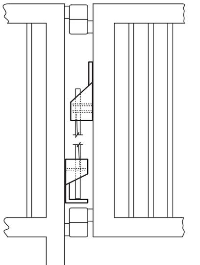
up to six torsion rods can be used for heavier gates
