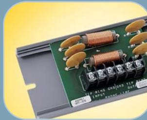
**surge protectors** are available for low voltage; high voltage and telephone line and help protect equipment from transient voltage spikes.
