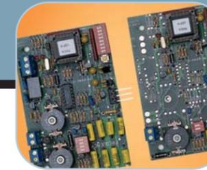
**plug-in loop detectors** simplify installation and are used for vehicle protection.
